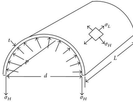
**Figure 3:** Hoop and longitudinal stress depicted on a visual model.
