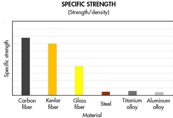
**Figure 1. Comparing the strength to weight of composites to metals.**
