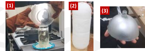
Figure 7: (1) Melting the wax used to create the mold for the pressure vessel (2) the solidified cylindrical mold made of wax (3) the metal washer unique to this design that adds structural stability
