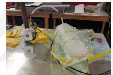
Figure 9: Curing the carbon fiber
